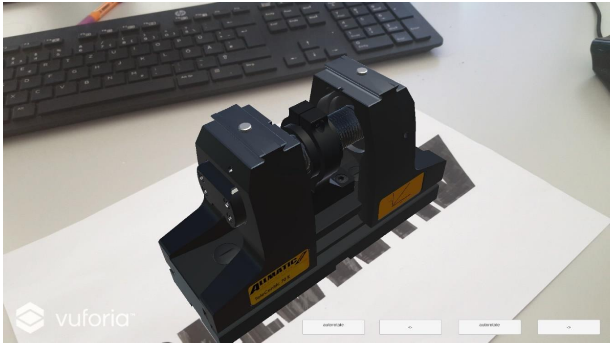
FIGURE 14 MARKER-BASED AUGMENTED REALITY WITH THE SOFTWARE “VUFORIA” IN THE GAME ENGINE UNITY
